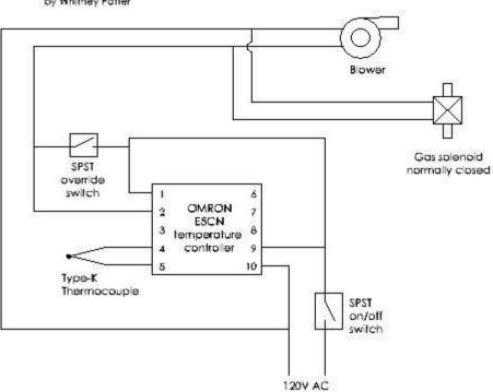
Temperature Controller Wiring Diagram
