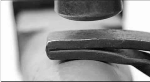
Nick and fold over the leaf and scroll assembly. Weld over the bick
