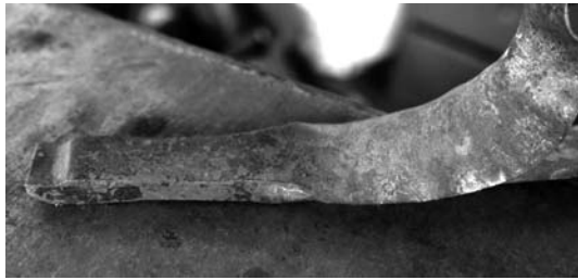
Correct orientation of scarf. This keep the leaf up and the scroll down making a more stable arrangement
